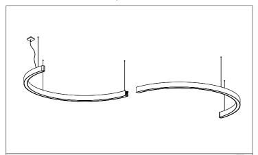
1. The luminaire must be installed in the order indicated on the labels, starting with parts A, B, C....
