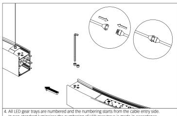
All LED gear trays are numbered and the numbering starts from the cable entry side.
